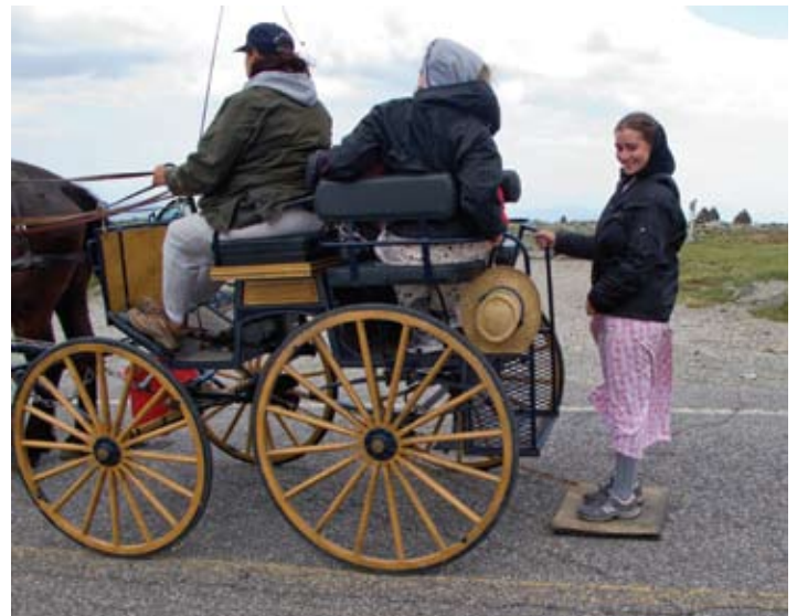
A high-tech braking system—a thick rubber mat chained to the carriage, with one or two passengers standing on it—eased the descent and spared the carriage brakes. Photo courtesy of Mount Washington Carriage Road.
